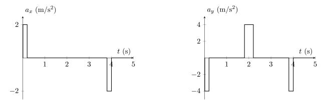
Sketch the **velocity** and **position** in the x and y directions from t = 0 s to t = 5 s. Label the **axes** with units and indicate the values at each of the **peaks**, **valleys**, and transition points in your plots (e.g., at t=0.2, 1.8, 3.8, 4, 5s). Feel free to sketch on a separate paper if easier.
